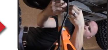
Attach headlight to wire harness as shown. Secure excess wire with zip ties.
