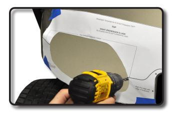
Cut out the shape of the headlight. Use the cutting tool to remove the excess trim. \*Flip template over repeat process on the other side.
