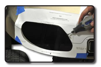
Use sandpaper to smooth out any rough edges. Mount headlight through the cutout. Push top half in first as shown.
