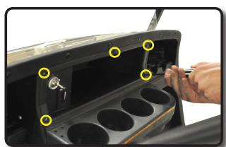
Using a 15/32" drill bit, drill out the hole for the rocker switch.\*Drill gently. Remove nut from rocker switch, feed switch through the drilled hole and tighten with nut.
