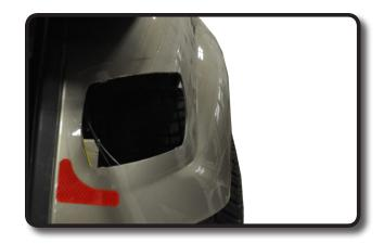
Feed the tail light harness through the back of the cart. Attach rear tail light wire harness as shown. Secure wire with ties.
