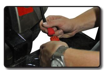
Place tail light into the rear of the vehicle. Insert four self tapping screws into tail light using supplied hardware.\*Repeat process on other side.
